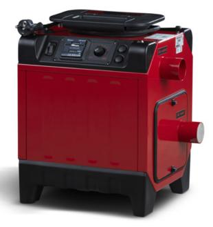
The small but powerful turbine has a capacity of up to 180 m<sup>3</sup>/h and a pressure of up to 260 mbar. The turbine's air volume/-pressure can be adjusted based on the drying assignment's size and demand. When the temperature rises, the output is regulated down. This is done so that the machine can continue to work even at extreme load and not stop and require manual resetting as several other machines on the market do.
