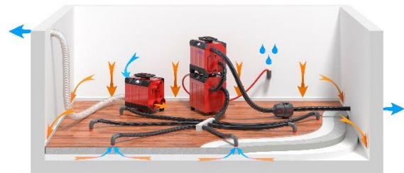
Suction drying. The dryer dries the ambient air and the turbine draws and evacuates air from the construction. The resulting underpressure in the construction draws dry air into it.
