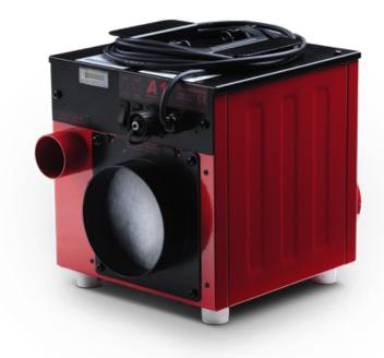
A1 is, like all Corroventa machines, a robust dehumidifier that can withstand tough environments. It is a simpler, compact and lightweight option that makes it easy to transport and handle. It is equipped with a multi-speed fan for optimal distribution of dry air. The dehumidifier is also equipped with hygrostat for energy efficient use, as well as an MID approved kWh meter.
