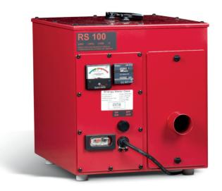
Radon extractor RS100 (turbine extractor) has been specially developed for radon remediation or negative pressure ventilation in buildings with foundation constructions of cellar, split-level or slab type. RS 100 has a high level of suction and is therefore particularly suitable because fill material under the building's base plate is expected to have relatively little air, creating large counterpressure. RS 100 is very quiet and can be installed in residential environments.
