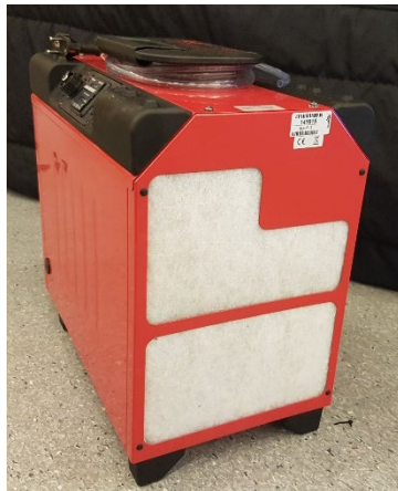
Process/cooling air inlet with filter
