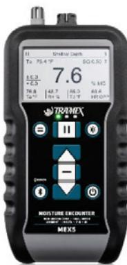
The Moisture Encounter MEX5 has a built-in hygrometer for ambient conditions and psychrometric values, an Infrared Surface Thermometer and also incorporates external in-situ RH probes for in-situ equilibrium RH readings, as well as Pin probes for wood, drywall, and WME readings. Moisture test results can be visualized and Geotagged with the Tramex Meters App and turned into moisture maps, reports and charts for sharing.
