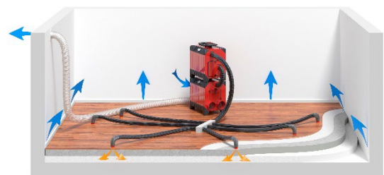
Pressure drying. The turbine is fed with dry air from the dehumidifier and presses this air into the layered construction.
